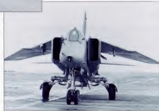
Below: The original MiG-27K 'Flogger-D' has now been supplanted in the Russian air force by the improved MiG-27M 'Flogger-J' and '-J2', with provision to carry more precision-guided munitions.
